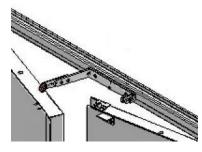
Mechanical device of high resitance and quality that allows the coordination in the closure of a door specially designed for evacuation of buildings and/or fire resitance doors
